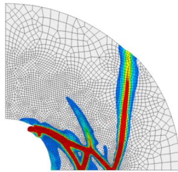
(b) Adaptive refinement in the zones of high shear strain localization
