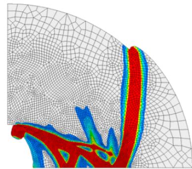
(c) Simulation subsequent to gross collapse through adaptive remeshing
