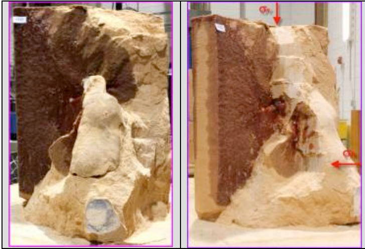
Figure 6 - Experimental results of the test performed in a Saltwash Red sandstone block with a wellbore inclination \alpha = 45^\circ , azimuth \beta = 90^\circ , and anisotropic far-field stress \sigma_v = 2,400 psi, \sigma_H = 1,560 psi, \sigma_h = 1,040 psi. Multiple transverse and parallel fractures are initiated in this configuration.
