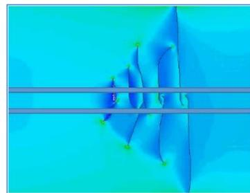
Multi-well fracture interference (plan view)
