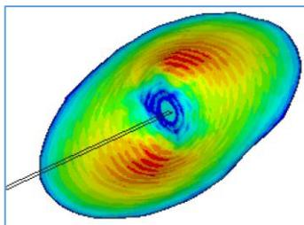
Fracture curving in 3D (contours showing aperture)
